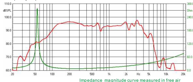
Frequency response measured in a closed enclosure of 600L in an anechoic chamber
